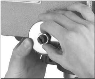
Figure 43. Loosening cover and jam nut
